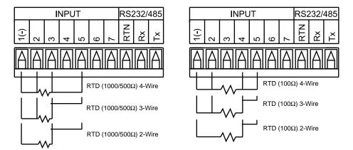
Figure 2.6 a) RTD-1000 ohm and 500 ohm Wiring Hookup
